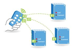
The receivers will be controlled simultaneously. Maximum 4 receivers. Unlimited number with "Radio bus" (see § B-1)
