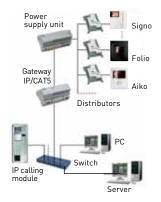
pag. 24 Advantages and applications: Two non-polarised wires THROUGHOUT for quick and easy installation. Ideal for villas and large residential complexes alike: 4 main entrances, 32 risers, 128 users per riser column for a total of 4096 users. Free intercom function with four monitors in parallel, integral video surveillance, second entrance management.
