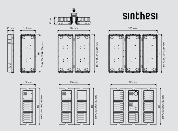
NOTE: H1 = 114, 204, 294, 384 indicates flush mounting height and H2 = 119, 209, 299, 389 indicates to total height relative to 1, 2, 3 and 4 module versions.
