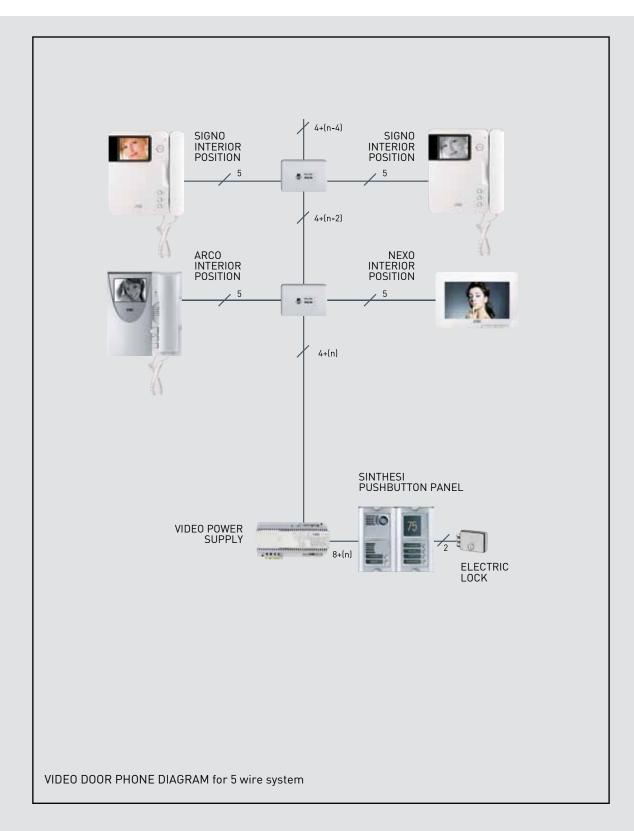
SINTHESI PUSHBUTTON PANEL: WITH COLOUR CAMERA FROM 1 TO 20 BUTTONS (SIGNO COLOURS, NEXO)
